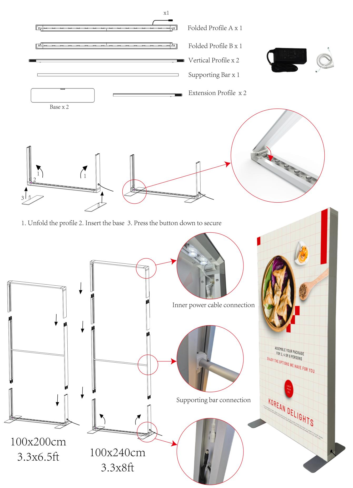
Inner cable and power supply connection
