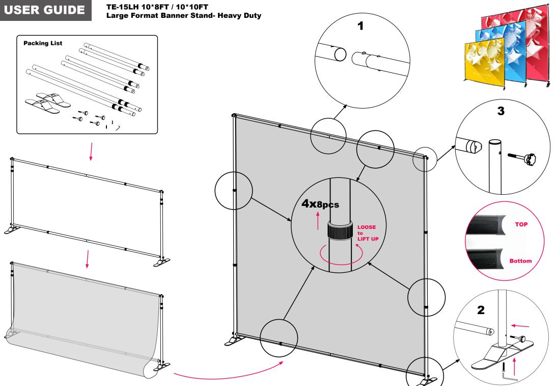
After installing the hardware and printing, adjust the frame to the suitable size.
